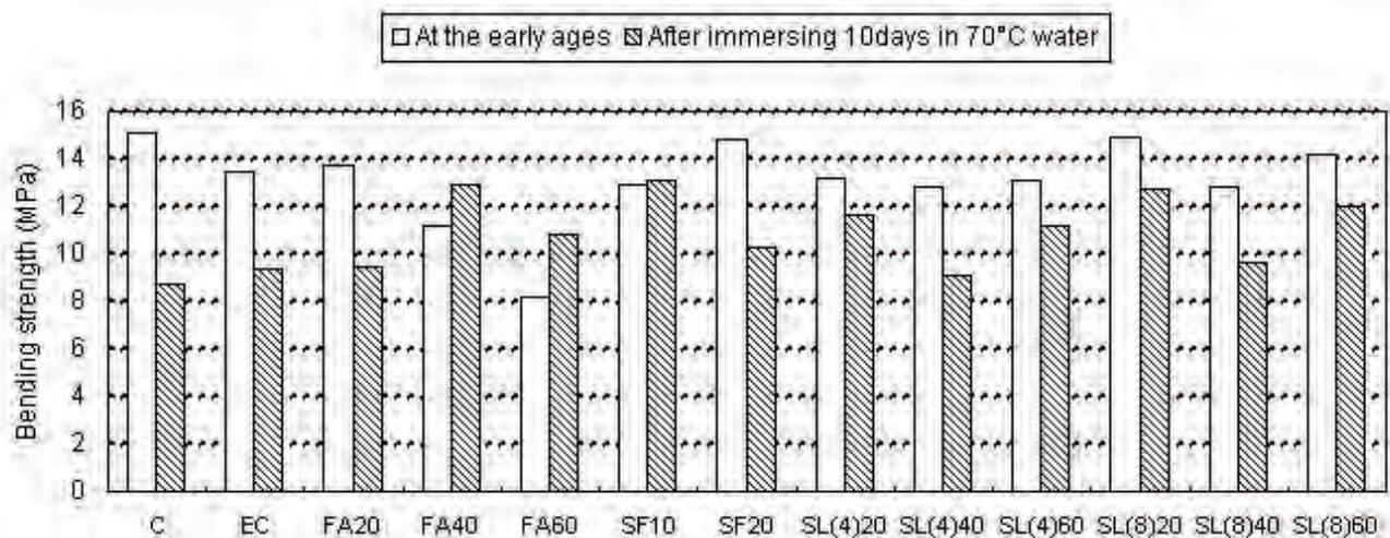
Figure 2 - Bending strengths before and after accelerated aging
