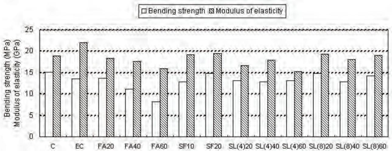
Figure 1 - Bending strength and modulus of elasticity at early ages
