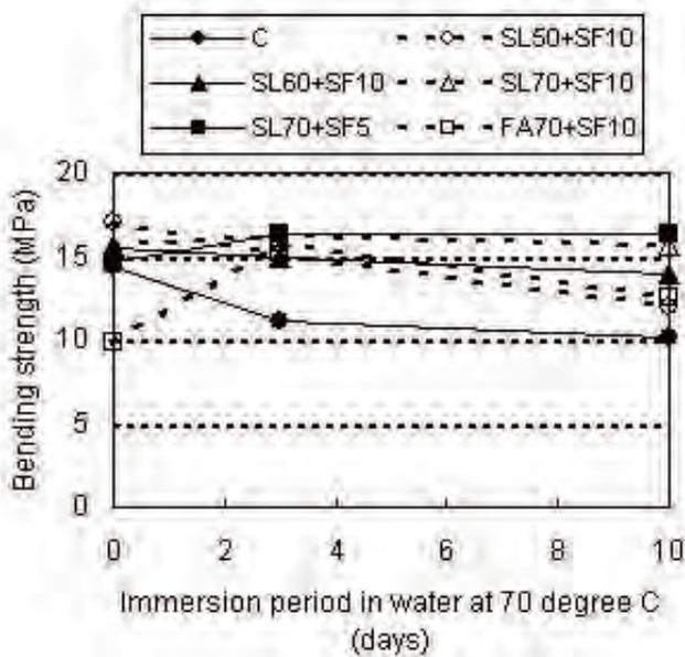
Figure 3 - Bending strength
