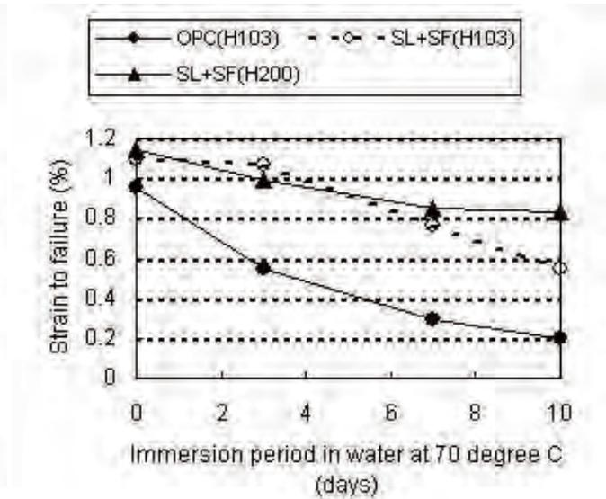
Figure 6 - Strain to failure
