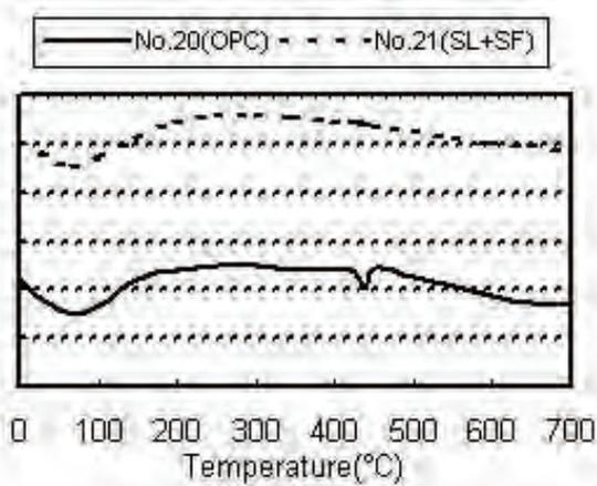
Figure 7 - DTA of hardened mortar
