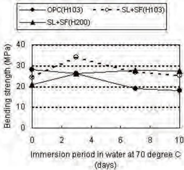
Figure 5 - Bending strength
