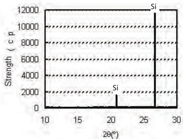
Figure 9 - XRDA of hardened mortar (No. 21: SL+SF)
