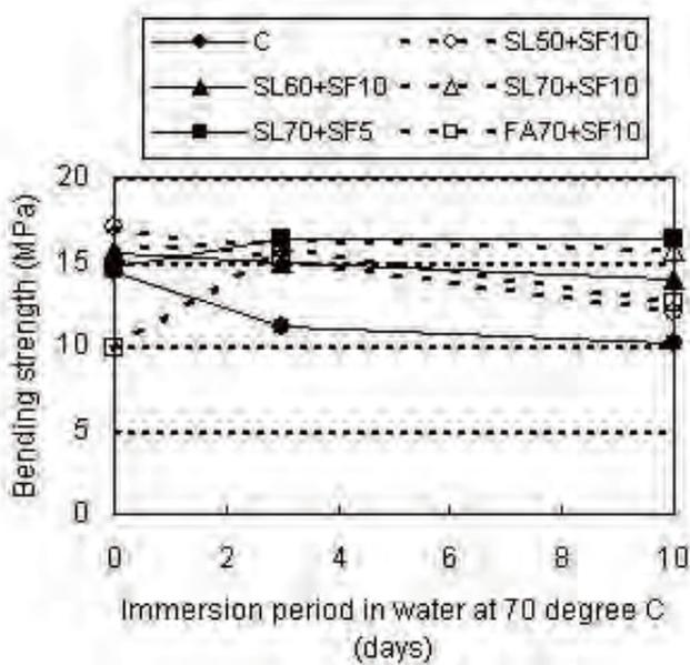
Figure 3 - Bending strength
