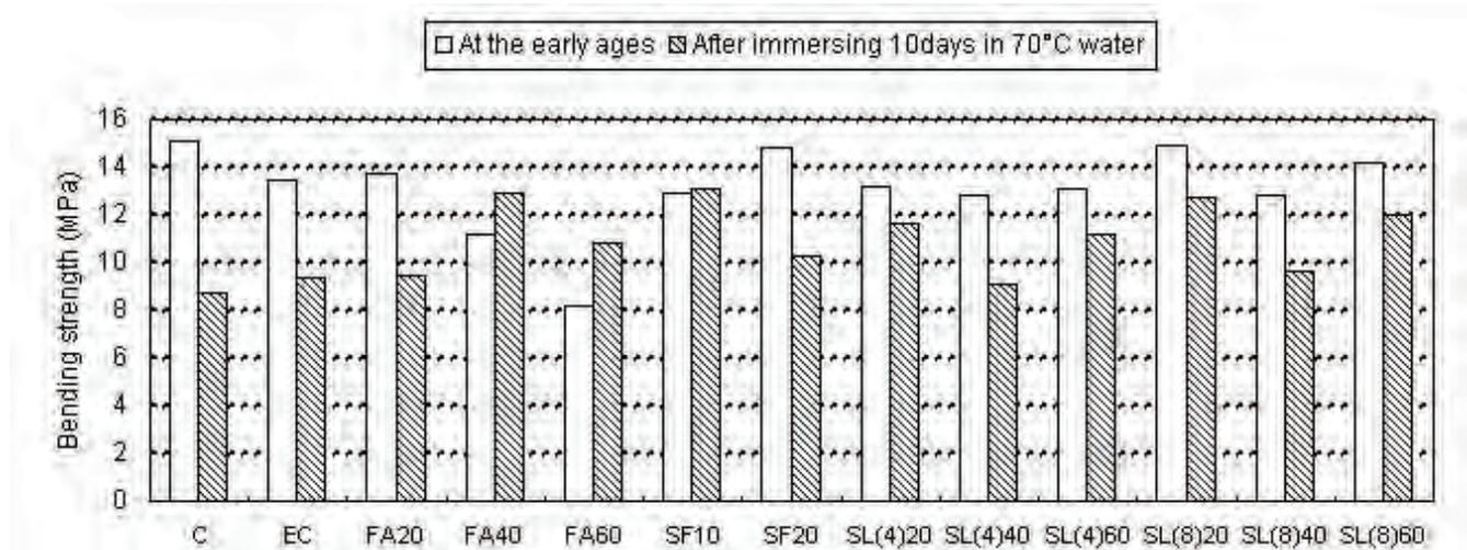
Figure 2 - Bending strengths before and after accelerated aging
