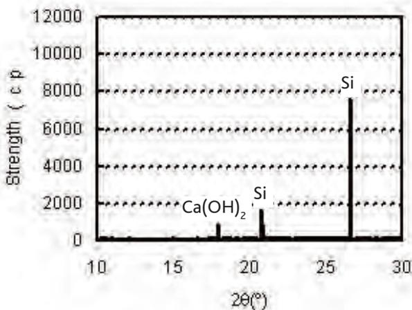
Figure 8 - XRDA of hardened mortar (No. 20: OPC)
